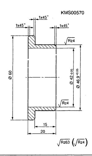
Centering sleeve for pulling deep-groove ball bearing off intermediate bearing:
